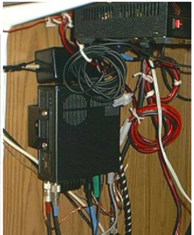
My latest bedside operating desk. Middle shelf slides out for use. 706 head mounted underneath top shelf on PanaVise cell phone mount.
